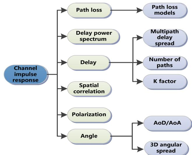
Figure 3: Typical parameters for characterizing the MIMO channels
