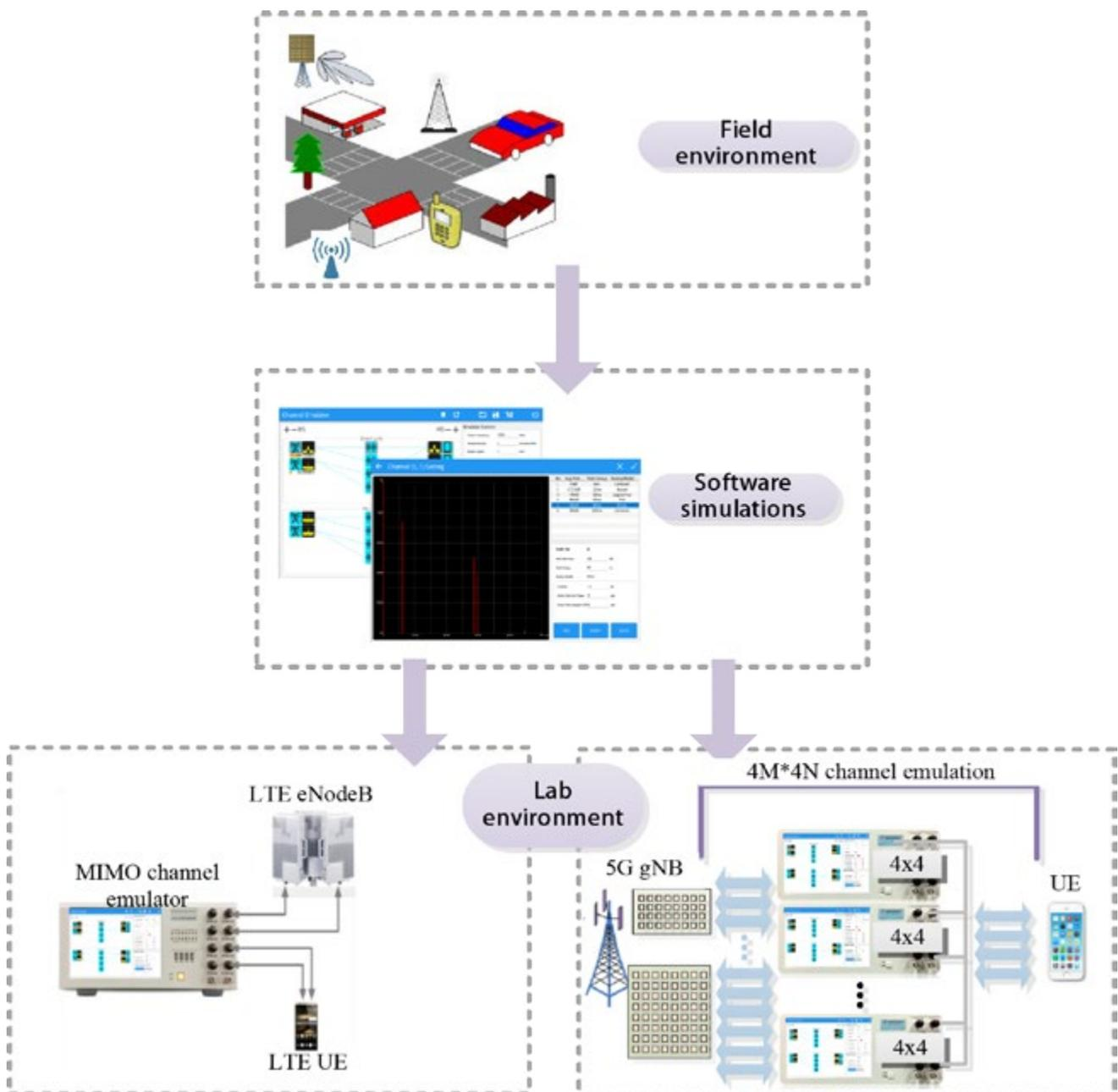
Figure 5: Setup of test systems with the channel emulator
