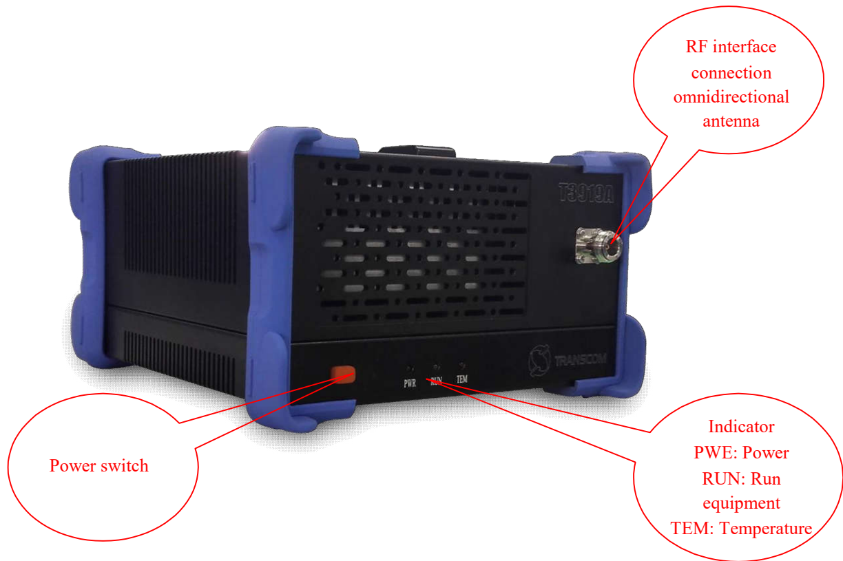
Fig. 1 Front Connection of Transmitter
